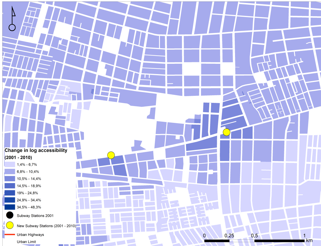
Figure A2: Change in log accessibility (2001 - 2010) - Close-up of the west of Santiago's subway network.
